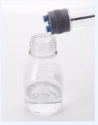
⑤ Open the caps and remove washing solution through syringe port.
