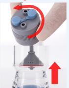
① Turn the volume control handle in count clockwise to lift the holder up to the point, "stop".
