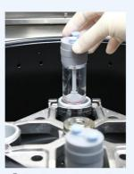
③ Put the tube in centrifuge and put the balance tube at count part. Then, centrifuge it at 1500rpm for 5 minutes.
