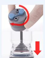
4 Turn the volume control holder to 4mL\* Open both of tube caps
