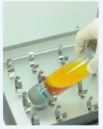
② Mix the fat with enzyme using Shaking Incubator with setting 37℃ and 150rpm for 30~40minutes.
