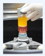
3 After completing tissue dissociation, measure the weight of 1st tube and get a balance tube ready with same weight for balance. Then, centrifuge the tube at 1500rpm for 5 minutes.
